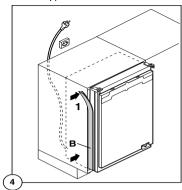
Screw appliance into place and retain the cabinet with screws (I) through the securing brackets into the worktop or adjacent woodwork as necessary.
